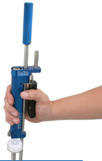
The SonTek deluxe wading rod, featuring a sturdy grip and bubble level.
